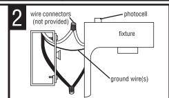
CONNECT THE WIRES. NOTE: Attach black fixture wire to black supply wire, white fixture wire to white supply wire. Do not mix them up. Use wire connectors (not provided). Connect bare fixture ground wire(s) to ground wire from outlet box.
