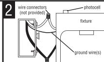
CONNECT THE WIRES. NOTE: Attach black fixture wire to black supply wire, white fixture wire to white supply wire. Do not mix them up. Use wire connectors (not provided). Connect bare fixture ground wire(s) to ground wire from outlet box.
