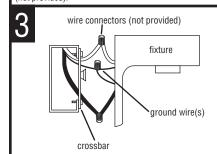
CONNECT THE WIRES. NOTE: Attach black fixture wire to black supply wire, white fixture wire to white supply wire. Do not mix them up. Use wire connectors (not provided) Connect bare fixture ground wire(s) to ground wire from outlet box. NEVER CONNECT GROUND WIRE TO BLACK OR WHITE POWER SUPPLY WIRES.
