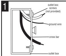
ATTACH the cross bar to the outlet box with outlet box screws (not provided)
